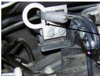
Ref. "B" (1) Throttle Cable Bracket (2) .636 long w/ 3/8" hole Spacers (2) 3/8-16 x 1 1/2" Bolts (1) Nutplate
